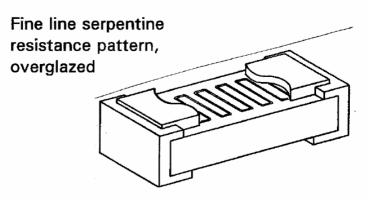
Sputtered Warp around termination: NiCr layer, Sn layer, solders: (lead free or 62-38)
