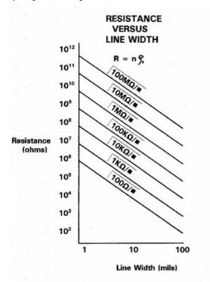
Figure 2 Resistance versus Line Width
