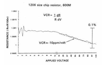
Figure 5 Variation of Resistance with Applied Voltage
