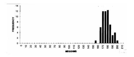
Figure 4 As Fired Resistance Distribution. 1206, 600MΩ
